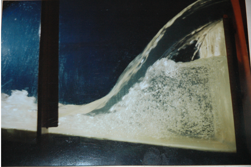
Fig. 2: The highly aerated circulating flow in the pool downstream a drop with negative sloping apron.
